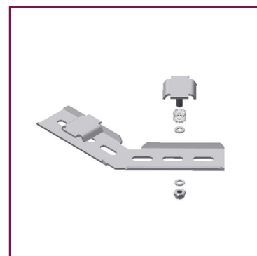
Mounting bracket 45° to connect 45° bends, side length 103x103 mm with 6 slotted holes 7x20 mm, completely assembled with clamping pieces, springs, washers and locking nuts
