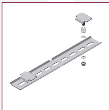
Bendable connector for individual connection of C-grid cable trays, length 264 mm with 9 slotted holes 7x20 mm, completely assembled with clamping pieces, springs, washers and locking nuts
