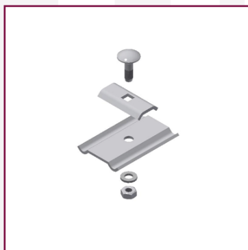
Side connector for a straight connection of C-grid cable trays, dimension 60x41 mm, completely assembled with truss-head screw, washer and nut
