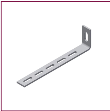
Fixing bracket no. 910, size 8 mounting element for universal use, dimension 215x25x55 mm, thickness 4 mm, with 5 slotted holes 6.6x26 mm and 1 slotted hole 11x26 mm
