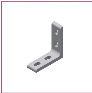
Fixing bracket no. 998, size 40 mounting element for steel channel 65 mm, dimension 120x40x120 mm, thickness 13 mm, with 4 slotted holes 14x25 mm
