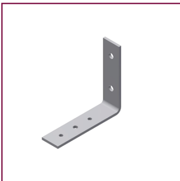
Fixing bracket no. 590, size 8 mounting element for universal use, dimension 119x30x108 mm, thickness 4 mm with 3 holes 2x 6 mm, 1x Ø 7 mm and 2 holes Ø 9 mm
