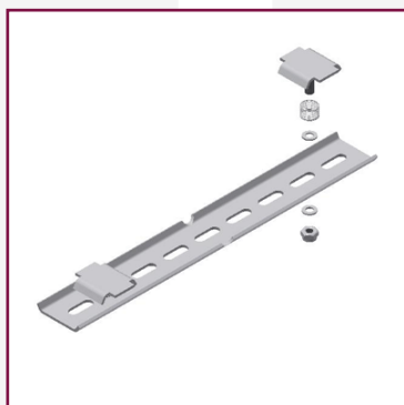
Bendable connector for individual connection of C-grid cable trays, length 264 mm with 9 slotted holes 7×20 mm, completely assembled with clamping pieces, springs, washers and locking nuts
