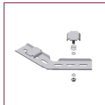
Mounting bracket 45° to connect 45° bends, side length 103×103 mm with 6 slotted holes 7×20 mm, completely assembled with clamping pieces, springs, washers and locking nuts
