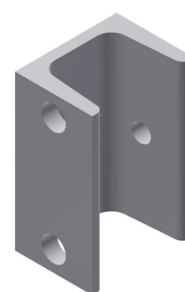
Mounting element for mounting the luminaire on the threaded pipe, made of steel channel 50×76 mm
