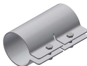
Connecting clamp DN65 Length 145 mm, for outer pipe diameter 76.1 mm, made of steel sheet 2.5 mm thick, with 2 hexagon screws M8×25, 2 hexagon nuts M8, 2 galvanised spring washers
