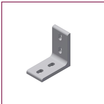
Fixing bracket no. 999, size 65 mounting element for steel channel 65 mm, dimension 120×65×120 mm, thickness 13 mm, with 4 slotted holes 14×25 mm
