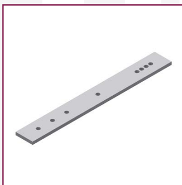
Mounting part, size 1 for protective pipe installation on sectional beams, length 245 mm, made of flat steel 30×5 mm, to be bent at the grain
