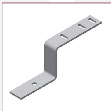
Mounting part universal piece for attaching junction boxes to the baseboard of grating platforms, made of strip steel 30×4 mm
