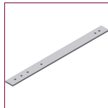
Mounting part, size 6 for protective pipe installation on sectional beams, length 385 mm, made of flat steel 30×5 mm, to be bent at the grain
